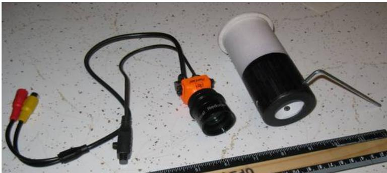
further in than is required by most all eyepieces - and the stronger the telecompressor, the more "in" focus is required. This can present a problem, especially for reflectors. When using the Night Eagle Astro camera, this extender tube is also useful in very cold temps as the end extending out of the telescope can be "plugged" lightly with a cloth, and the heat generated by the camera will keep the camera from getting "too cold" -
